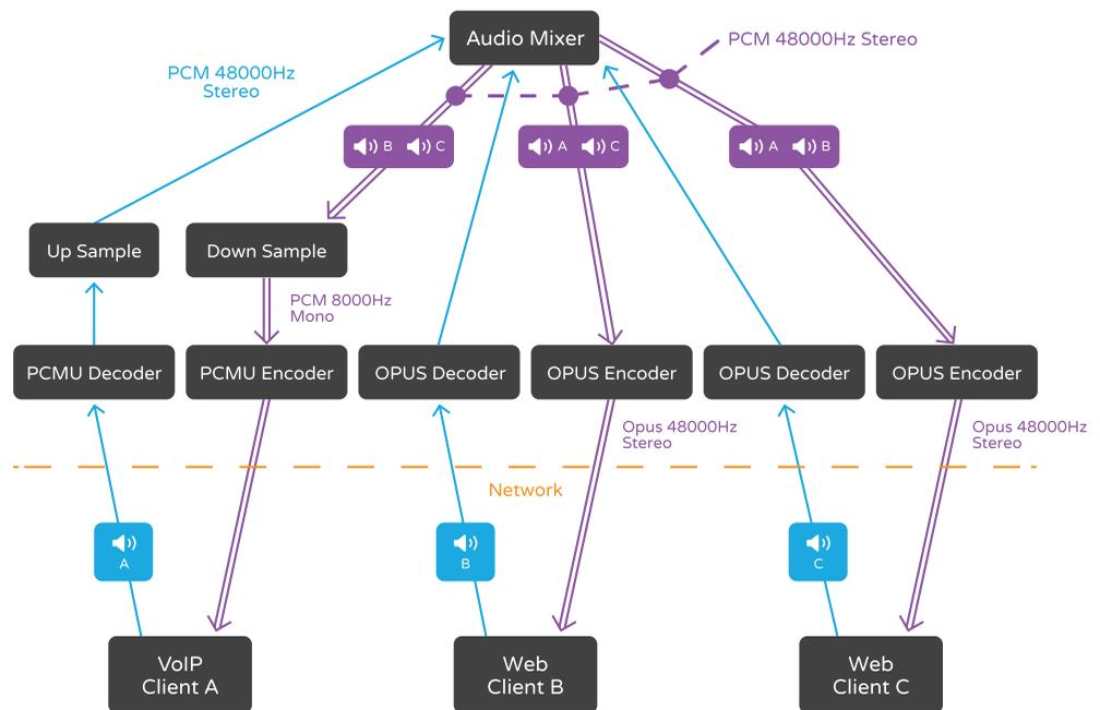
The SIP connector included with LiveSwitch ensures that both inbound and outbound SIP connections are MCU-based to avoid any potential compatibility issues with WebRTC clients. This allows LiveSwitch-based applications on desktop, mobile, and web to use the latest technology and highest-quality codecs available while allowing any number of legacy VoIP devices to join in.
